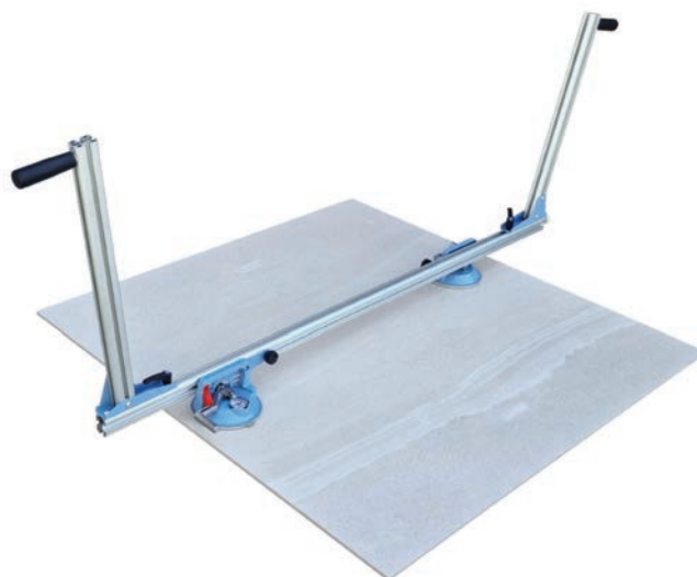
ERGO LIFT For handling and laying of tiles from 60x60cm up to 180x80cm Ideal for 2cm and 3cm thick outdoor porcelain pavers Load capacity 150 kg
