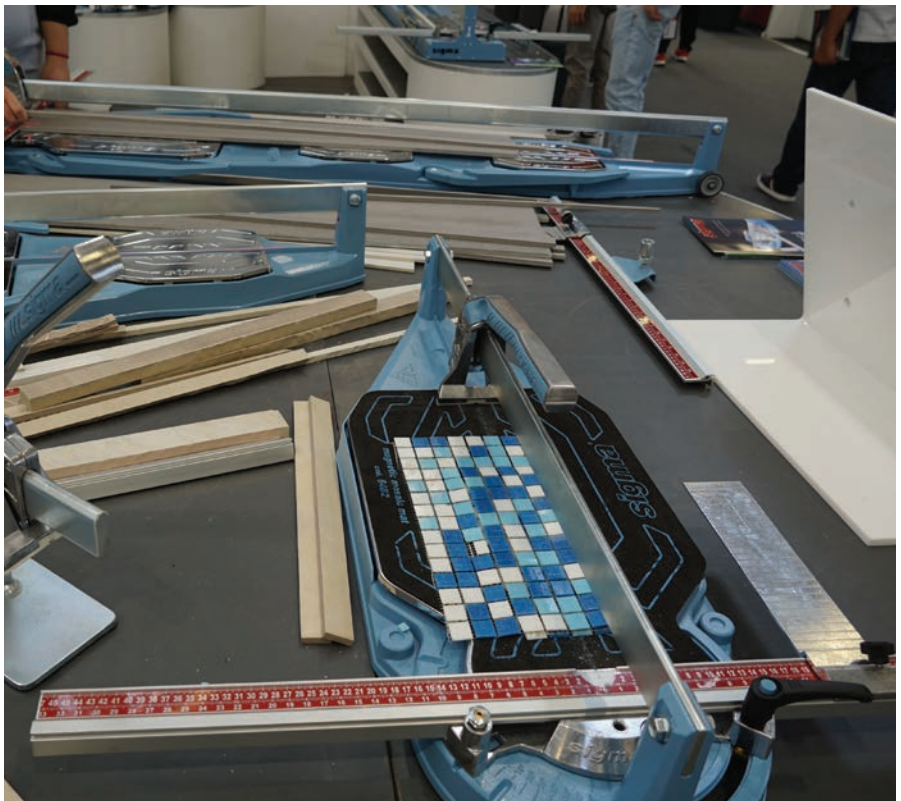
Sigma's non-slip Magnetic Mat non-slip is for mosaic cutting, and compatible with all Series 4 models Sigma
